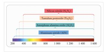
▲ Figure 1. Next generation optical waveguide platforms and wavelength transparency based on the bandgap ( $Si_3N_4$ ,  $Ta_2O_5$ ,  $Al_2O_3$ , and AlN)<sup>[49]</sup>
