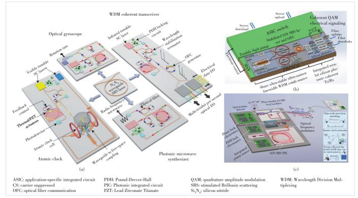
▲ Figure 6. Applications of SBS laser: (a) chip-scale atomic clock, integrated laser optical gyroscope, WDM coherent transceiver, and low-noise, photonic microwave synthesizer<sup>[71]</sup>, (b) example applications in coherent optical communication<sup>[93]</sup> and (c) optically synchronized precision fibre link<sup>[94]</sup>
