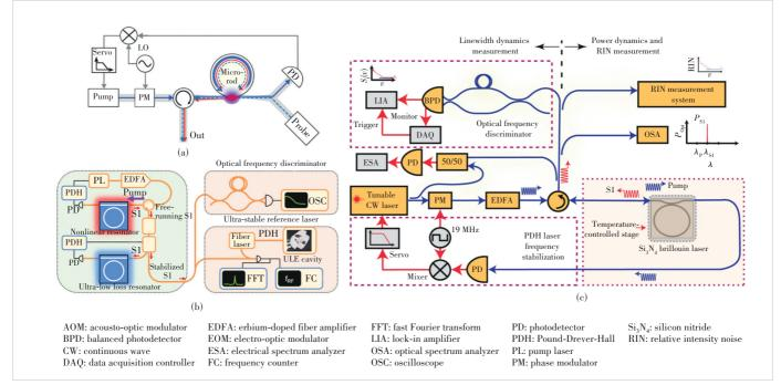
**\blacktriangle** Figure 5. (a) Measurement setup of Brillouin laser loaded  $Q^{[68]}$ ; (b) Brillouin laser stabilization and frequency noise measurement<sup>[90]</sup>; (c) measurement setup of Brillouin laser linewidth, phase noise, relative intensity noise (RIN) and power dynamics<sup>[71]</sup>
