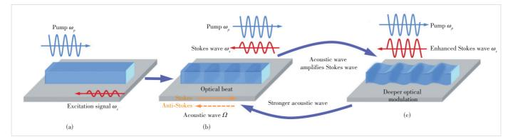
**\blacktriangle** Figure 2. Stimulated Brillouin scattering: (a) an optical pump interacts in the medium with a counterpropagating seed at the Brillouin frequency shift; (b) when the optical beat generated by said tones matches the Brillouin frequency shift, electrostriction induces an acoustic wave; (c) a stronger Stokes wave is created. The proposed deeper optical modulation generates a stronger grating<sup>[SS]</sup>
