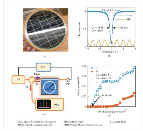
▲ Figure 4. (a) A 200 mm wafer after the manufacturing and dicing process; (b) resonance spectrum scan at 1 615 nm using a 1.078 MHz FSR Mach-Zehnder interferometer; (c) setup for the SBS laser; (d) measured on-chip power for S1 and S3 with the calculated curves, indicating a threshold of 0.38 mW<sup>[74]</sup>
